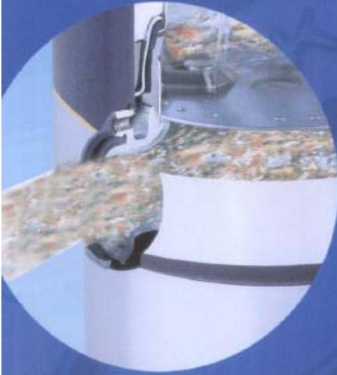
The ground waste is then flushed through the disposer tail pipe and the normal waste pipes to the water treatment plants. Here the waste is recycled into soil enhancement products or high combustion value fuel.
